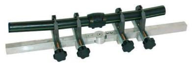
This professional tool is essential to hold pipes still and aligned during electrofusion. The **UNIVERSAL ALIGNER 63** is made almost entirely in a special Aluminium alloy and features a central joint for the fixed positions at 45° and 90°, four self-centring clamps that require no adapters. The possibility to remove one part of the axis that carries the clamps and one clamp it self, allows the use of tapping tees during the fusion.
